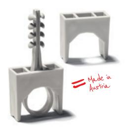
With the FS Fixing mounting base in connection with the DKS Dowel clamp, the effortless mounting of thermal conduction cables with a fixed distance of 8 or 15 mm to the ceiling is possible.
